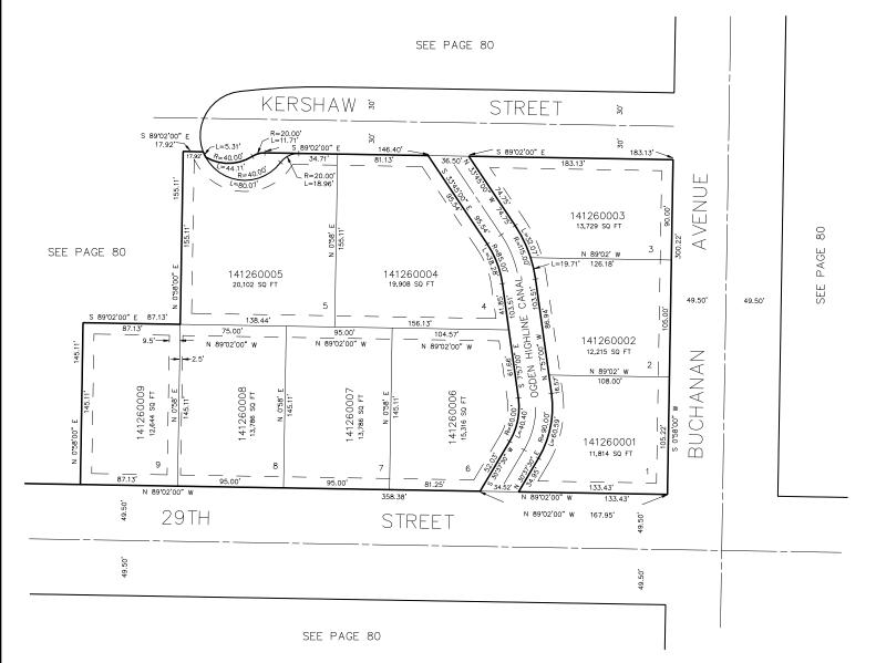
10' UTILITY & DRAINAGE EASEMENT EACH SIDE OF PROPERTY LINES AS INDICATED BY DASHED LINES EXCEPT AS OTHERWISE SHOWN.
